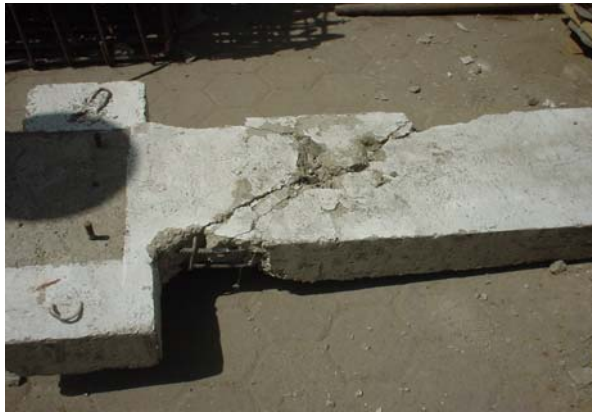
Figure 5 Failure of column C1
