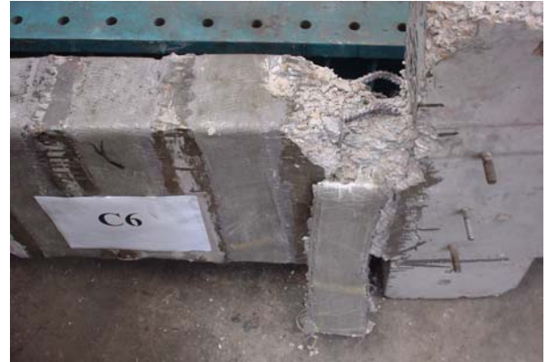
Figure 8 Failure of column C6
